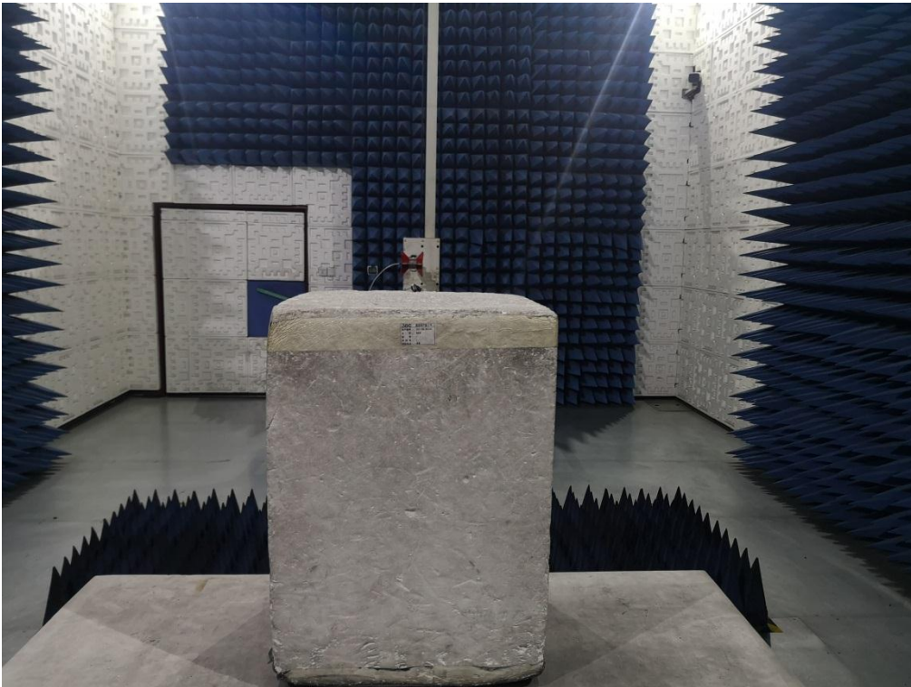
RADIATED EMISSION TEST SETUP ABOVE 1GHz
