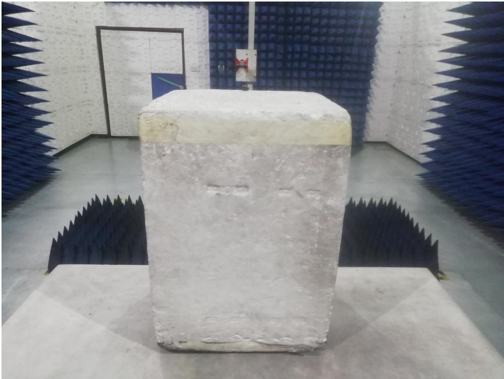
RADIATED EMISSION TEST SETUP ABOVE 1GHz
