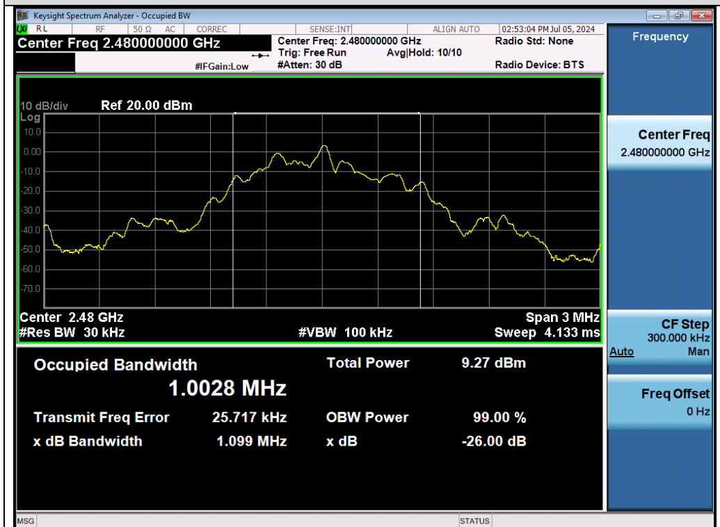
Test_Graph_LE1M_ANT1_2480_1Mbps_OBW
