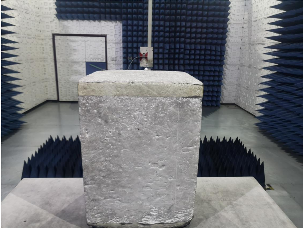
RADIATED EMISSION TEST SETUP ABOVE 1GHz
