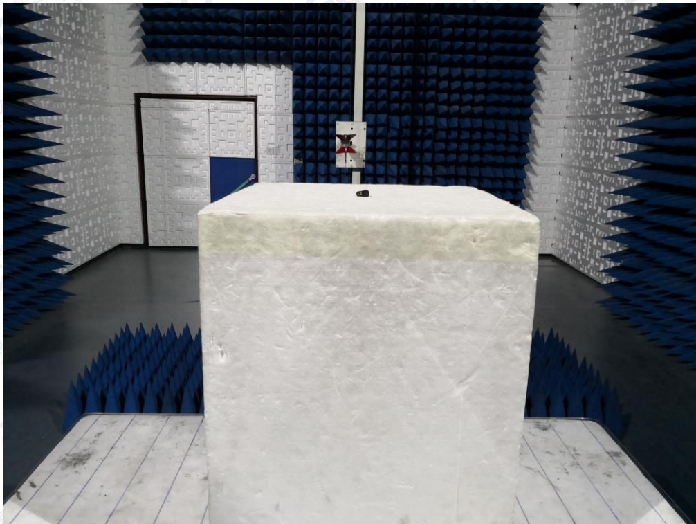
RADIATED EMISSION TEST SETUP ABOVE 1GHZ
