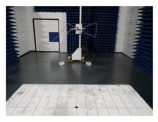
RADIATED EMISSION TEST SETUP ABOVE 1GHZ
