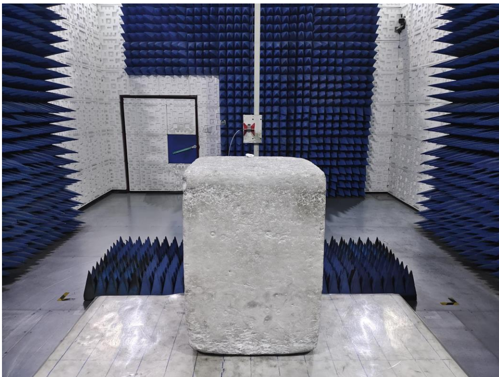
RADIATED EMISSION TEST SETUP ABOVE 1GHz
