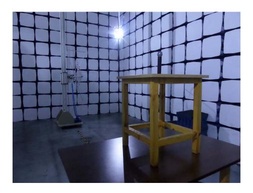
Radiation Emission Test Setup (Above 1GHz)
