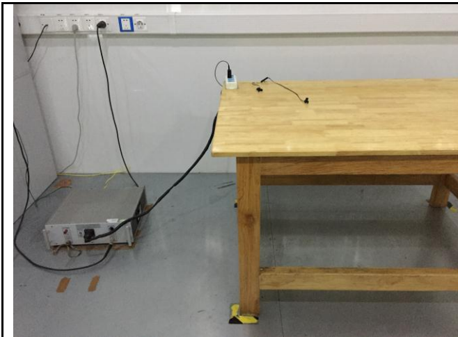
Conducted Emissions Test Setup Front View
