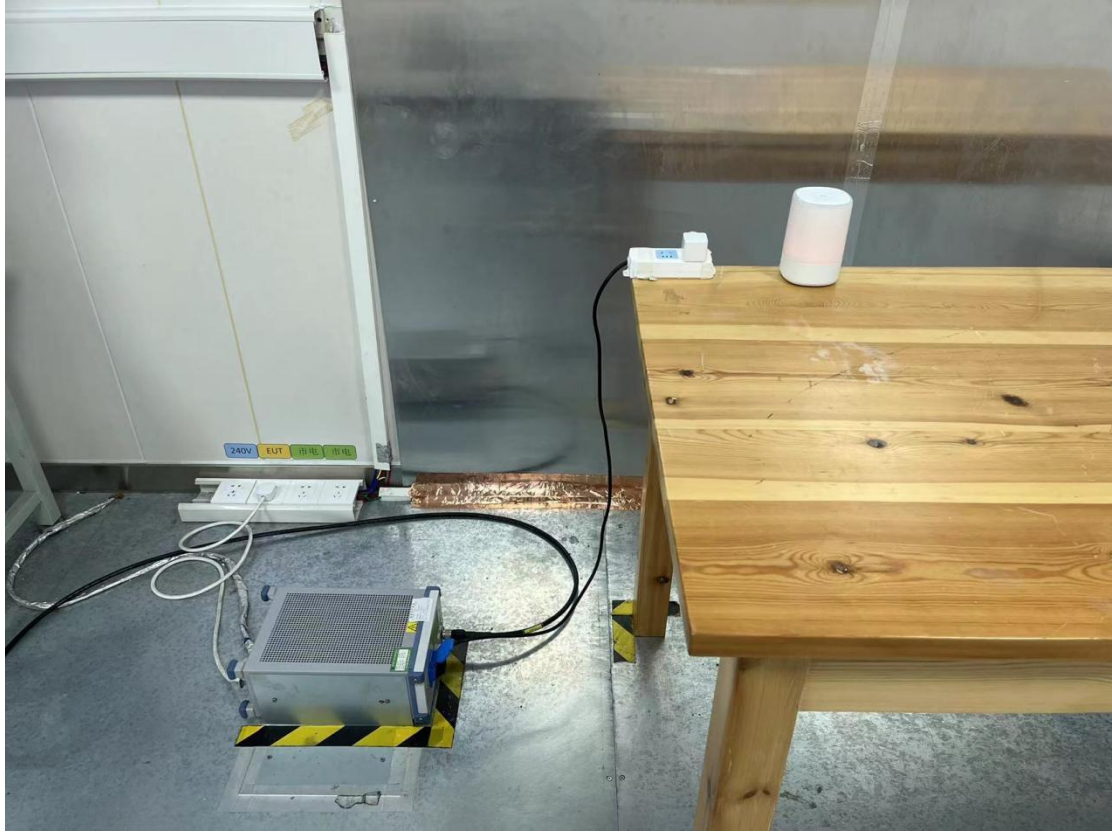
Conducted emission test setup
