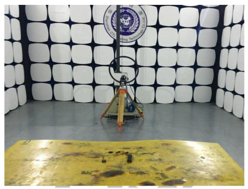
Radiated emission 30MHz~1GHz AI TESTING
