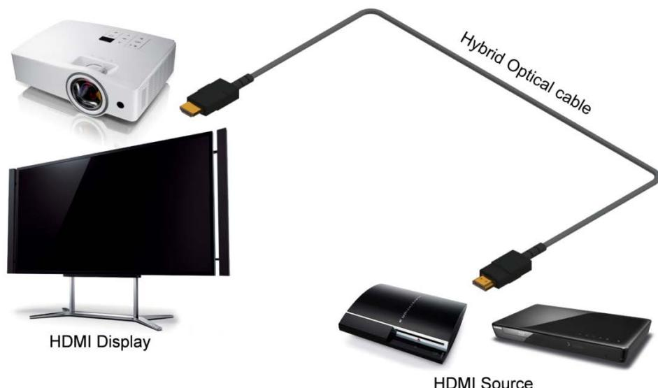
Please make sure that the direction of HDMI AOC connectors before connecting.
