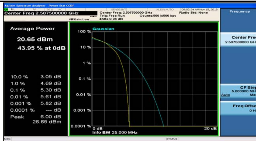
(Channel Bandwidth:15 MHz)_LCH_16QAM_37RB#38
