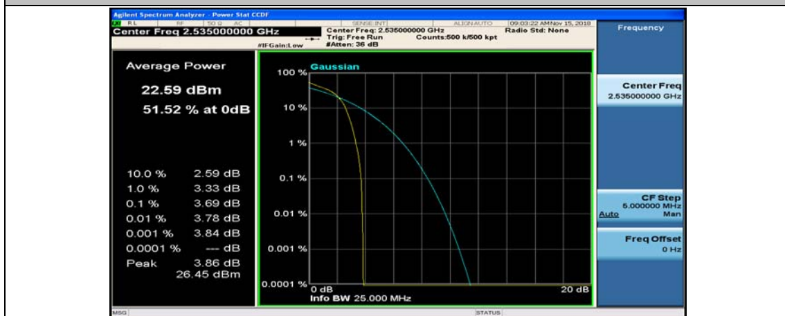
(Channel Bandwidth:15 MHz)_MCH_16QAM_1RB#74
