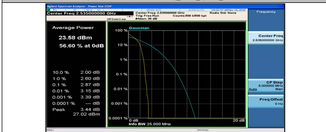
(Channel Bandwidth:15 MHz)_MCH_QPSK_1RB#37
