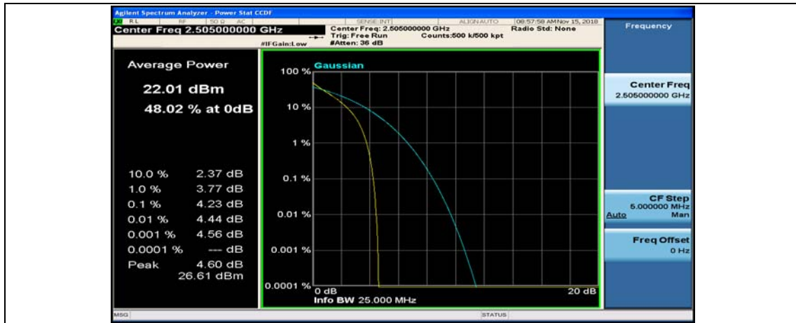
Channel Bandwidth: 10 MHz_MCH_QPSK_1RB#0
