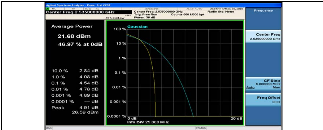
(Channel Bandwidth: 5 MHz)_MCH_16QAM_25RB#0
