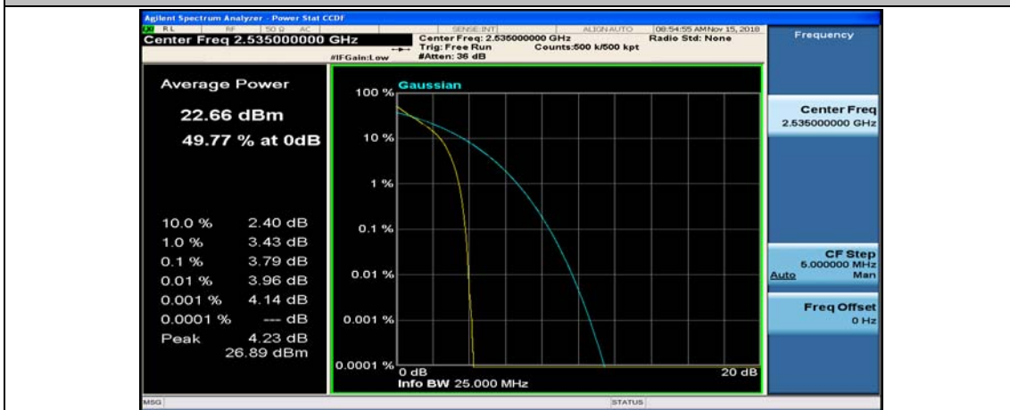
(Channel Bandwidth: 5 MHz)_MCH_QPSK_25RB#0
