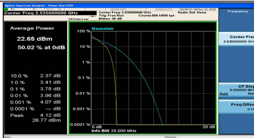
Channel Bandwidth: 10 MHz_MCH_QPSK_25RB#25
