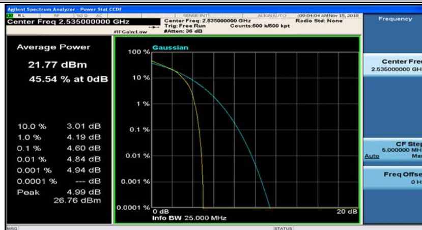
(Channel Bandwidth:15 MHz)_MCH_16QAM_37RB#38
