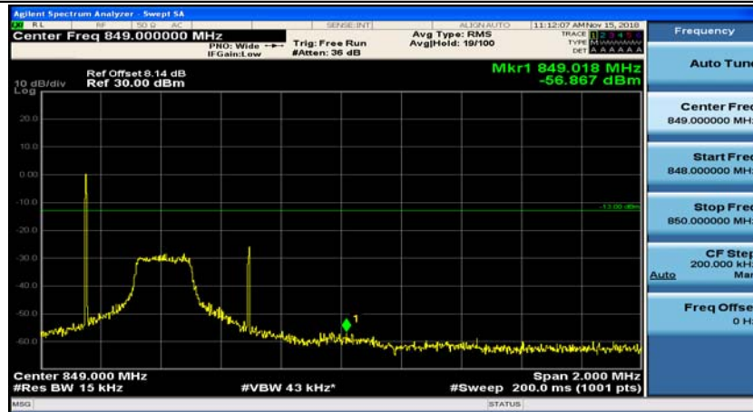
Channel Bandwidth: 10 MHz_HCH_16QAM_1RB#24
