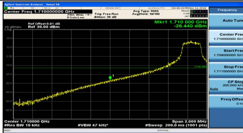
(Channel Bandwidth:15 MHz)_LCH_16QAM_1RB#37
