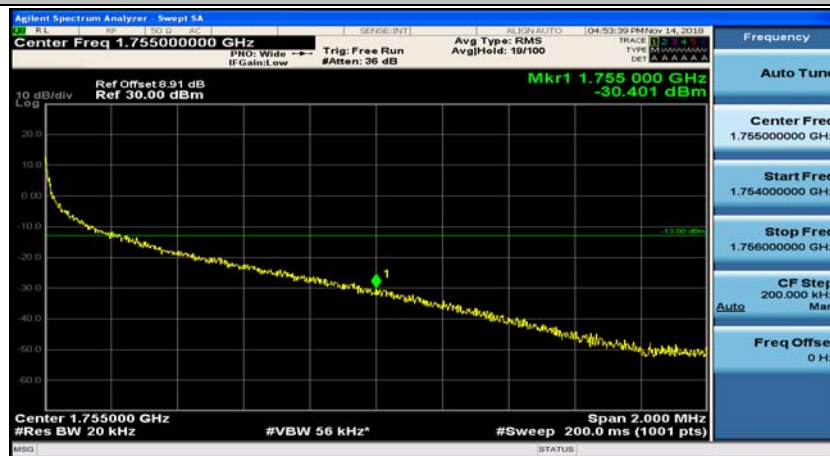
(Channel Bandwidth:20 MHz)_HCH_16QAM_50RB#0
