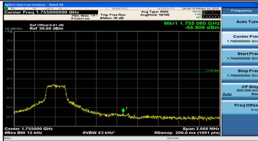
Channel Bandwidth: 10 MHz_HCH_16QAM_1RB#24
