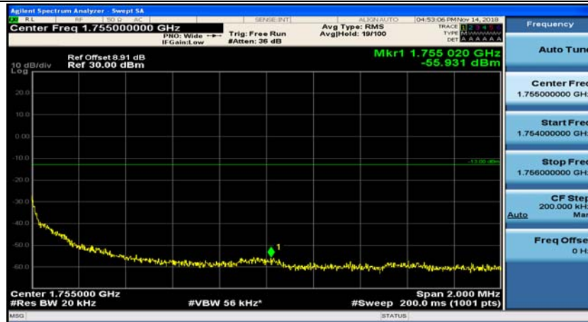
(Channel Bandwidth:20 MHz)_HCH_QPSK_1RB#49
