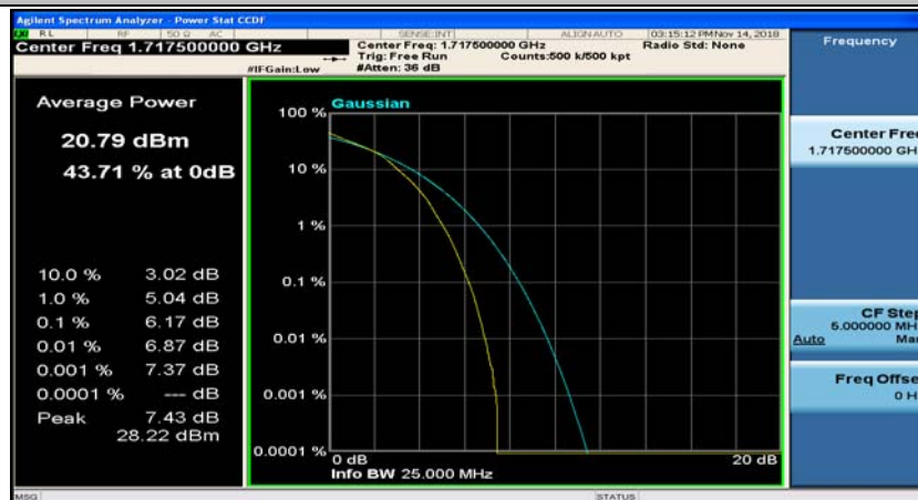
(Channel Bandwidth:15 MHz)_LCH_16QAM_75RB#0
