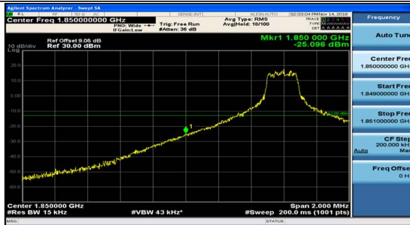
Channel Bandwidth: 10 MHz_LCH_QPSK_1RB#24
