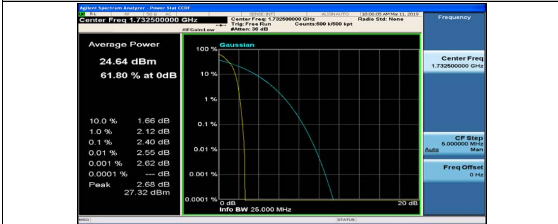
Channel Bandwidth: 10 MHz_MCH_QPSK_1RB#49
