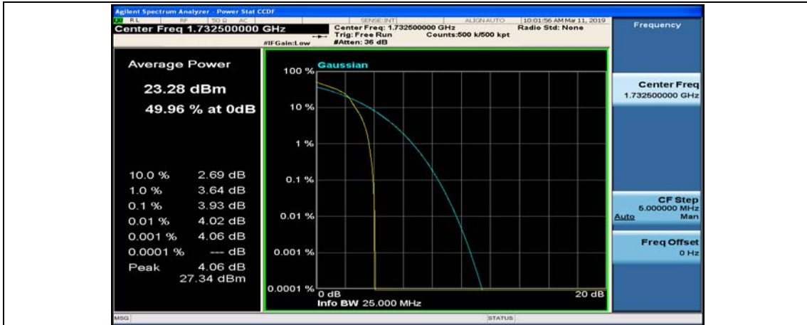
(Channel Bandwidth: 5 MHz)_MCH_16QAM_12RB#0
