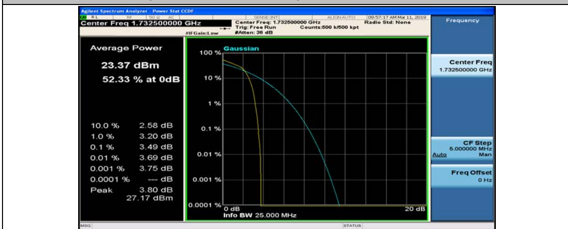
(Channel Bandwidth: 3 MHz)_MCH_16QAM_1RB#7
