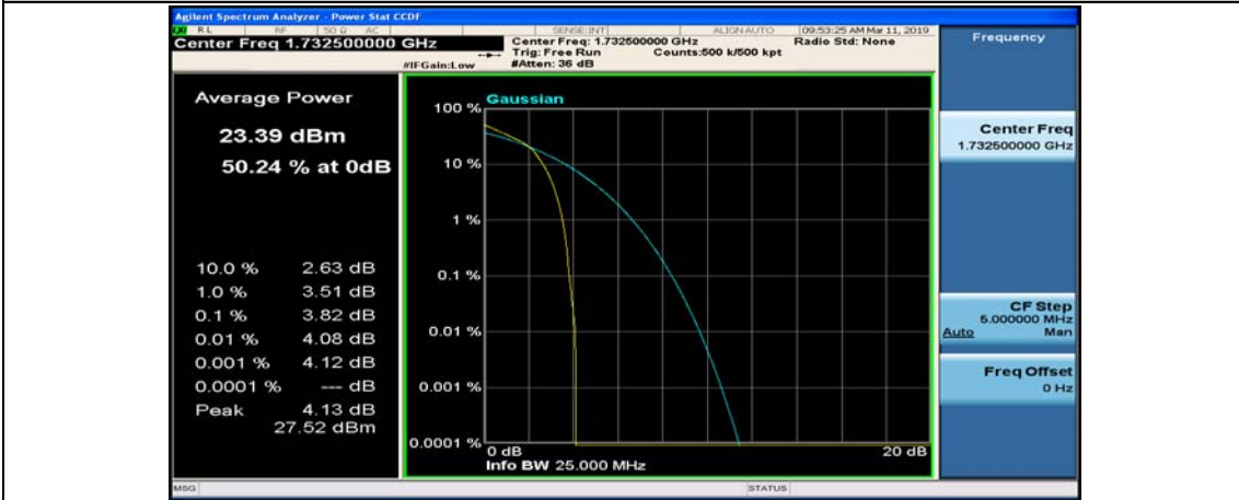
(Channel Bandwidth: 1.4 MHz)_MCH_16QAM_3RB#2
