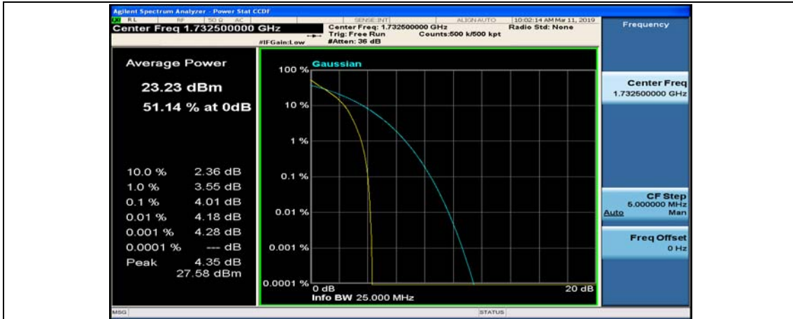
(Channel Bandwidth: 5 MHz)_MCH_QPSK_25RB#0
