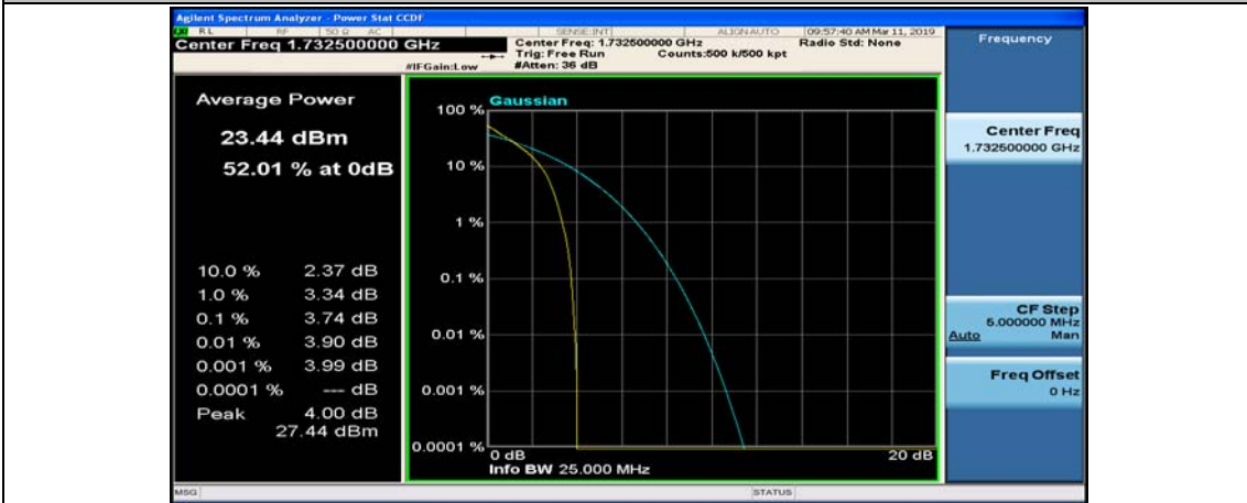
(Channel Bandwidth: 3 MHz)_MCH_QPSK_8RB#7
