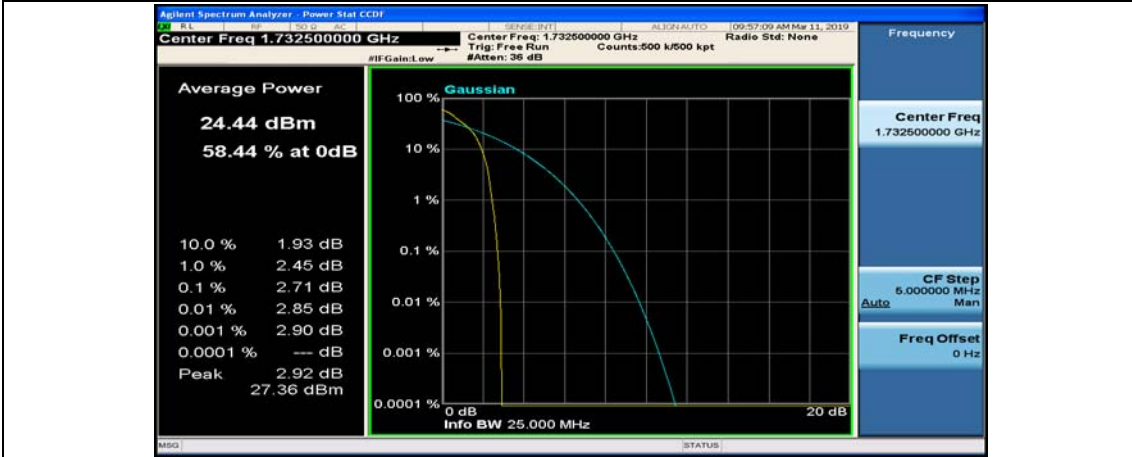
(Channel Bandwidth: 3 MHz)_MCH_QPSK_8RB#0
