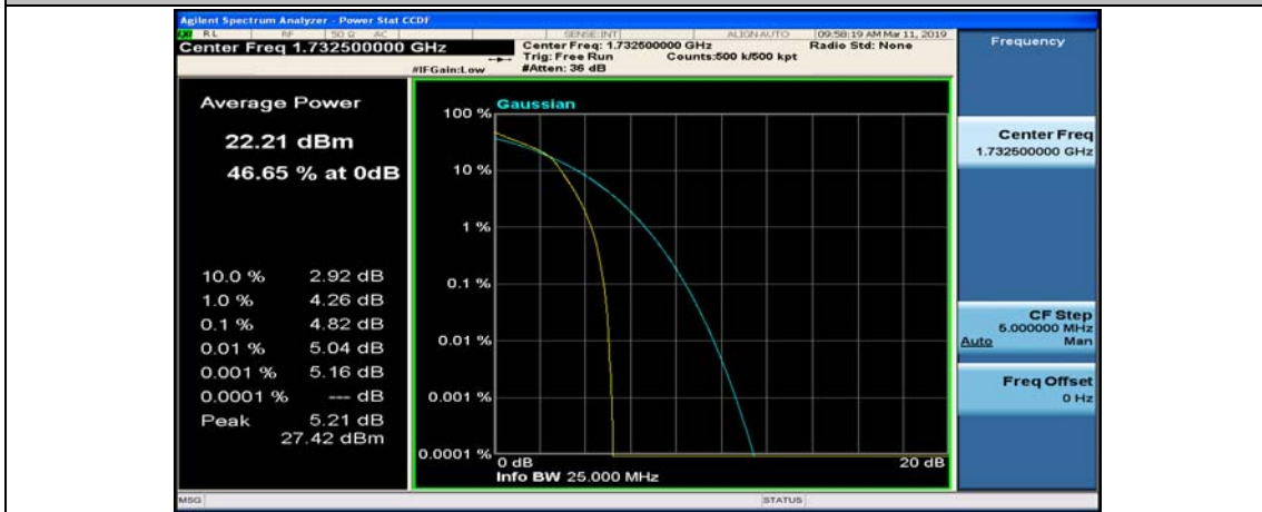
(Channel Bandwidth: 3 MHz)_MCH_16QAM_15RB#0
