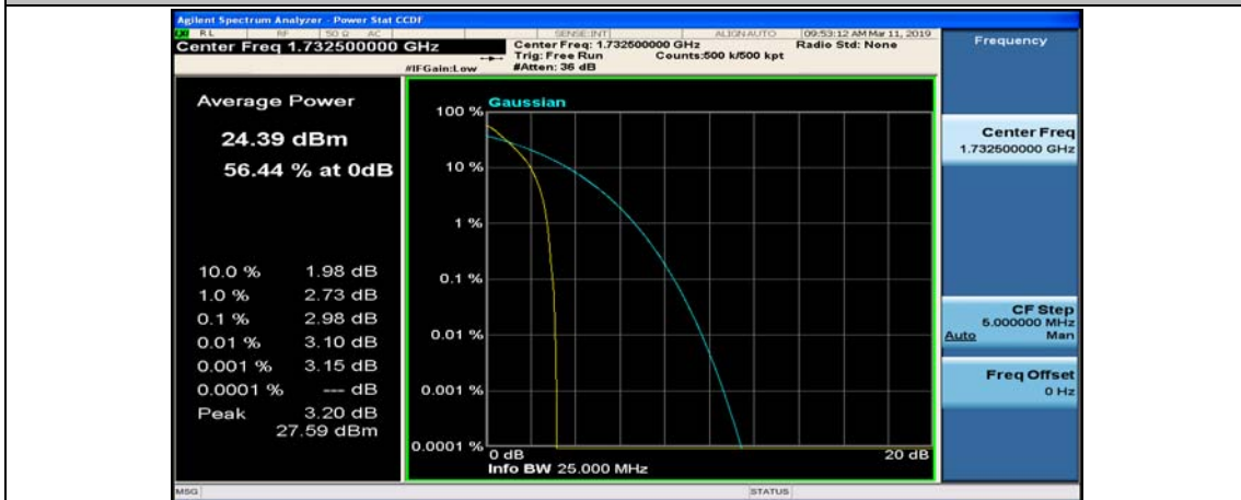
(Channel Bandwidth: 1.4 MHz)_MCH_QPSK_3RB#3
