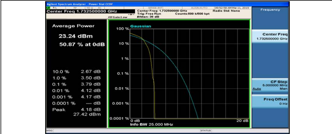
(Channel Bandwidth: 1.4 MHz)_MCH_16QAM_3RB#0
