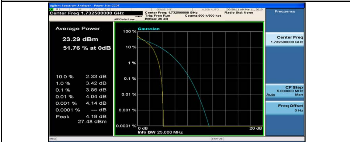
(Channel Bandwidth: 3 MHz)_MCH_QPSK_15RB#0
