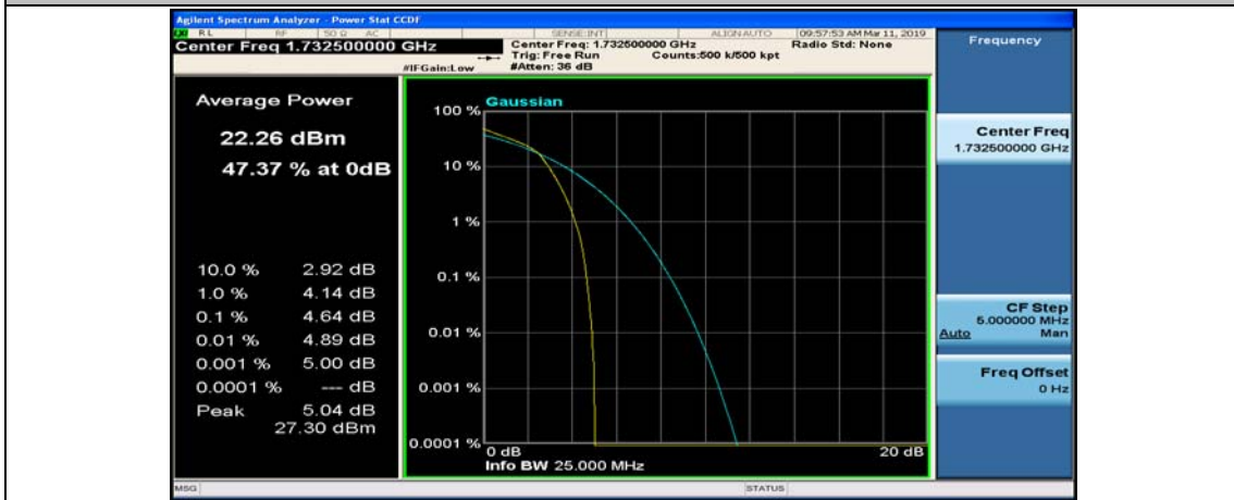
(Channel Bandwidth: 3 MHz)_MCH_16QAM_8RB#4
