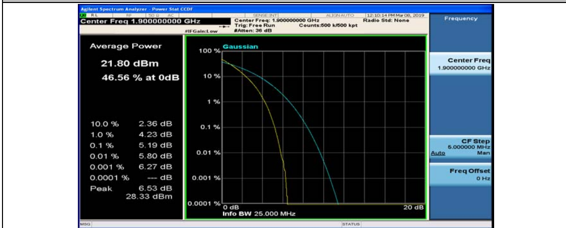
(Channel Bandwidth:20 MHz)_HCH_QPSK_100RB#0
