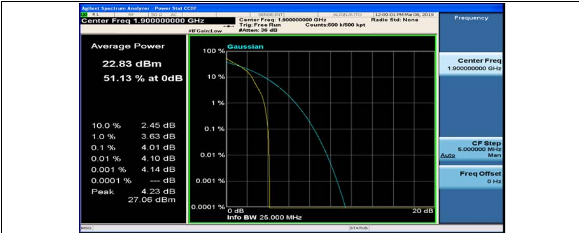
(Channel Bandwidth:20 MHz)_HCH_QPSK_1RB#99
