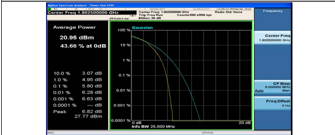
(Channel Bandwidth:15 MHz)_HCH_16QAM_75RB#0
