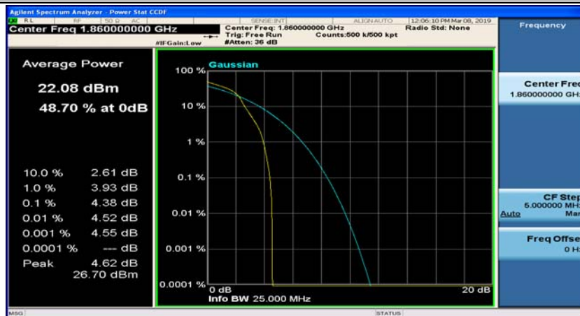
(Channel Bandwidth:20 MHz)_LCH_16QAM_50RB#0
