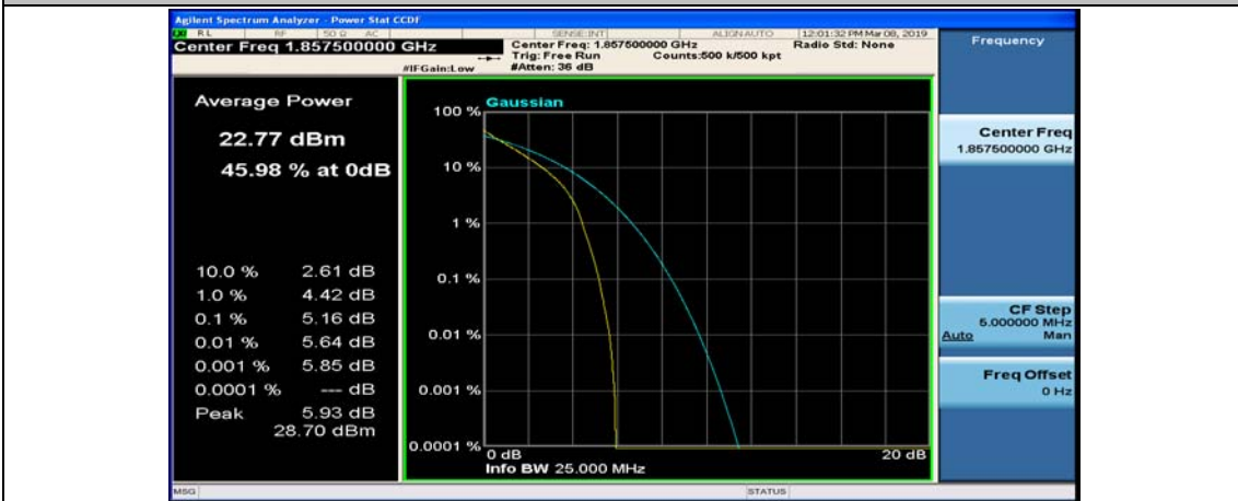
(Channel Bandwidth:15 MHz)_LCH_QPSK_37RB#38
