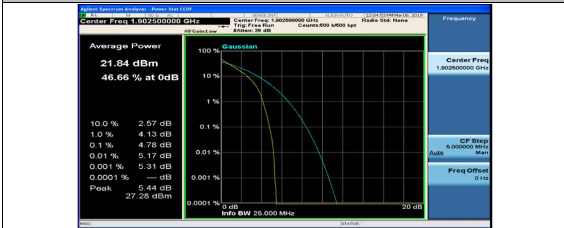
(Channel Bandwidth:15 MHz)_HCH_QPSK_75RB#0
