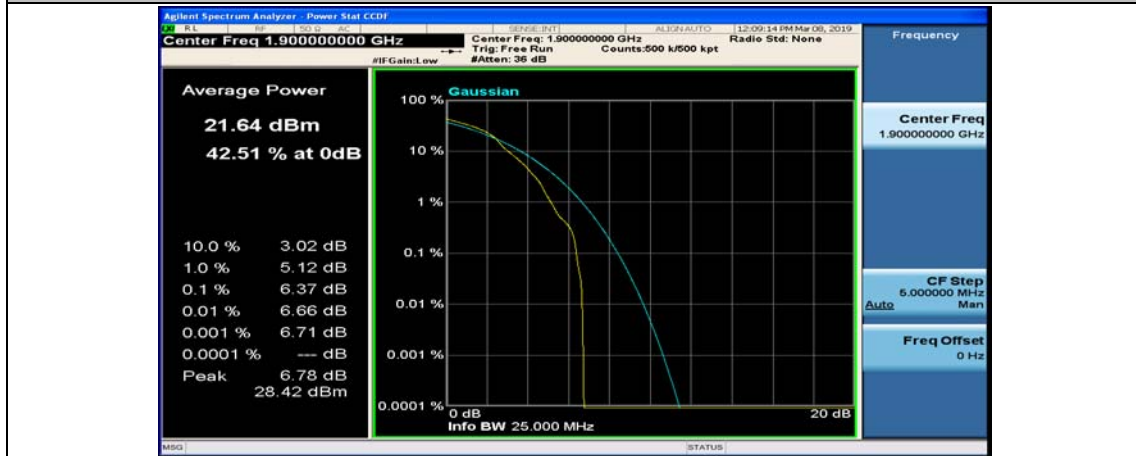
(Channel Bandwidth:20 MHz)_HCH_16QAM_1RB#49
