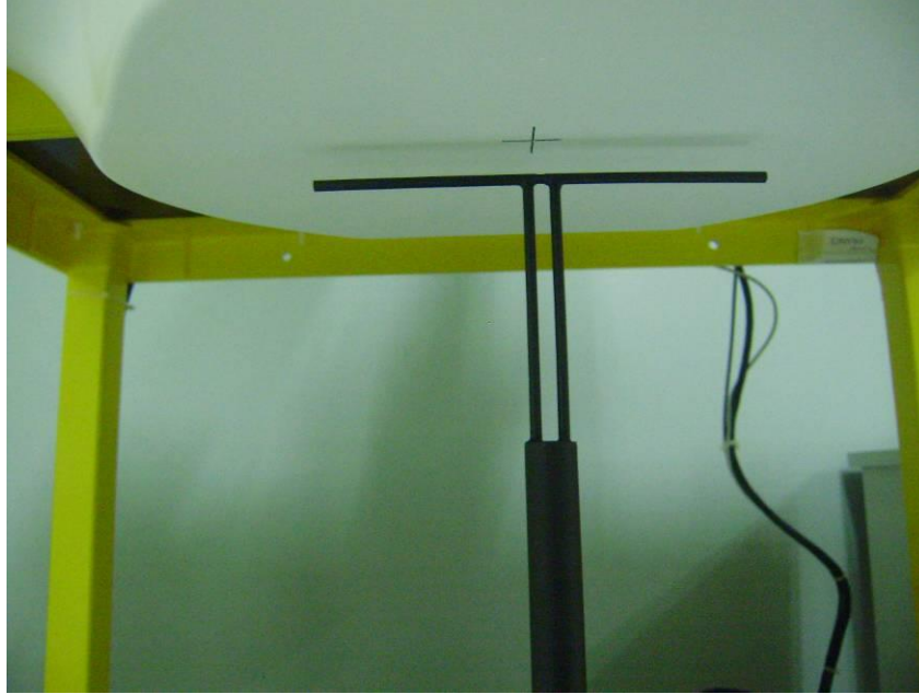
Setup Photo of Dipole Antenna
