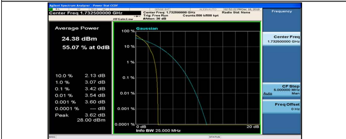
Channel Bandwidth: 10 MHz_MCH_QPSK_1RB#49
