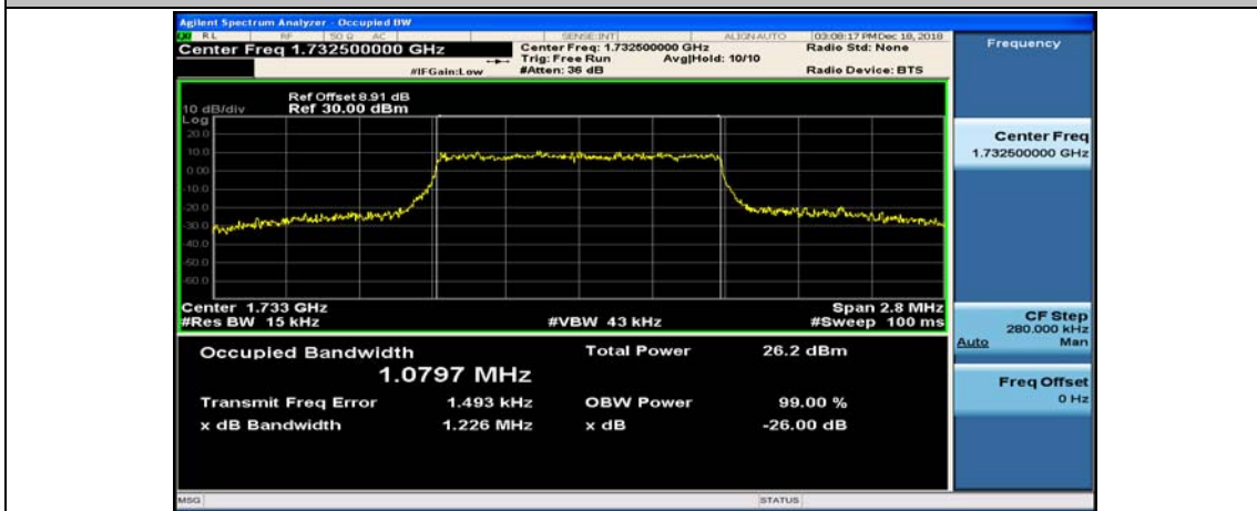
(Channel Bandwidth: 1.4 MHz)_MCH_16QAM_6RB#0
