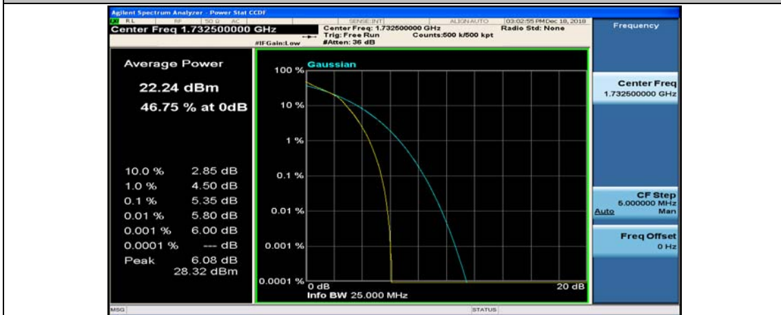
(Channel Bandwidth:20 MHz)_MCH_16QAM_50RB#50
