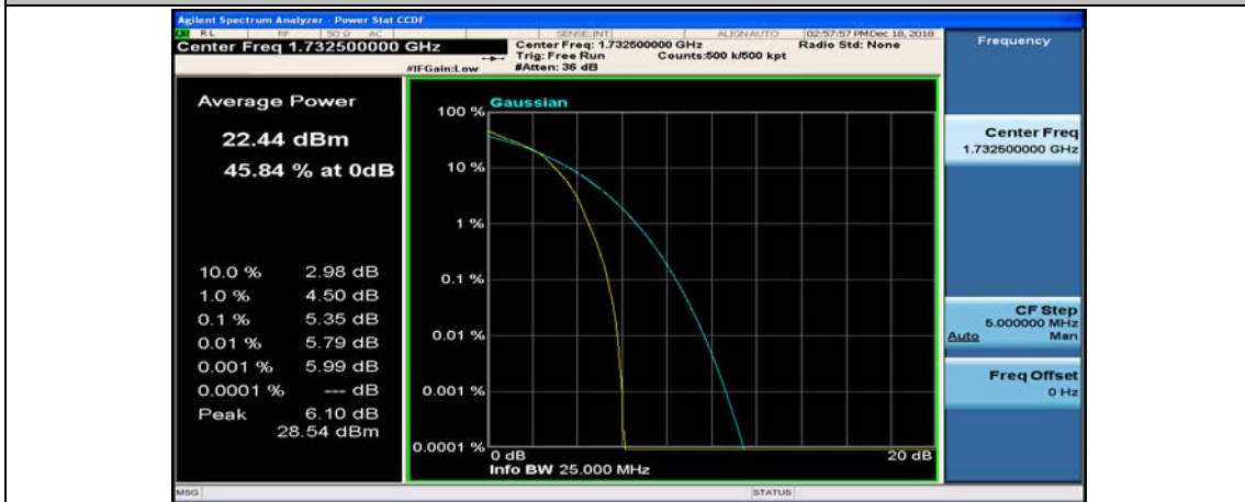
(Channel Bandwidth:15 MHz)_MCH_16QAM_37RB#18
