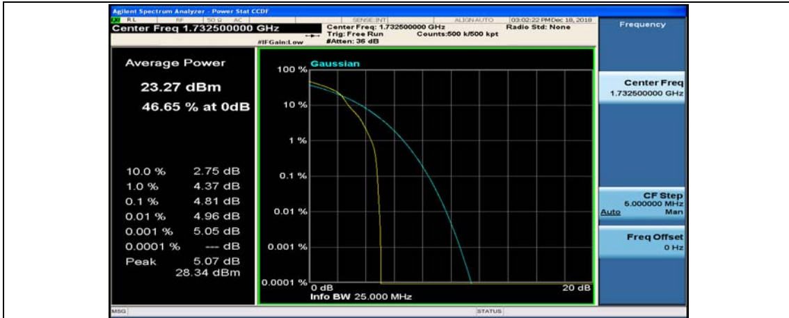
(Channel Bandwidth:20 MHz)_MCH_16QAM_50RB#0
