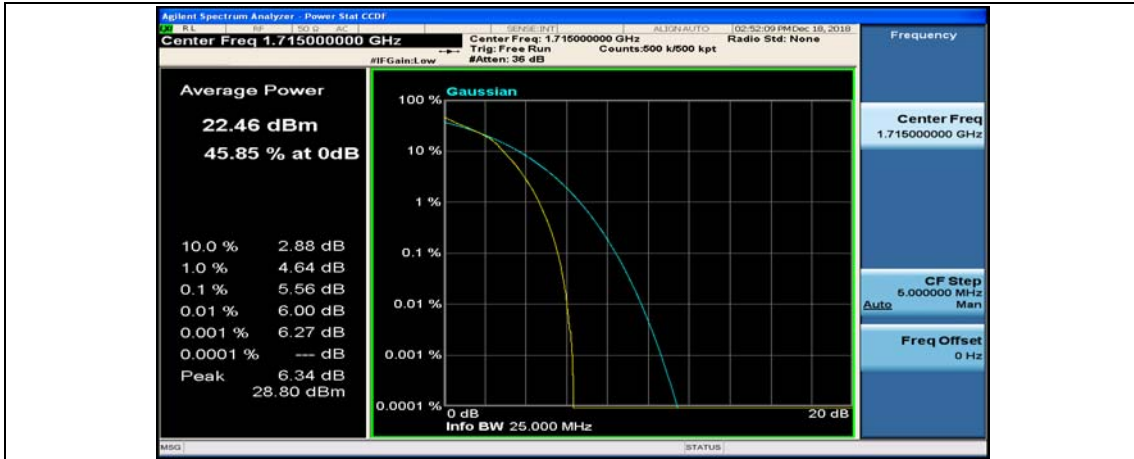
Channel Bandwidth: 10 MHz_MCH_16QAM_1RB#0
