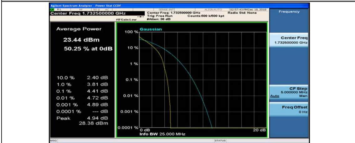
(Channel Bandwidth:15 MHz)_MCH_QPSK_37RB#38
