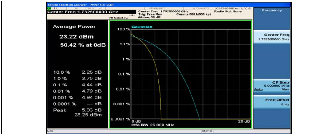
Channel Bandwidth: 10 MHz_MCH_QPSK_50RB#0
