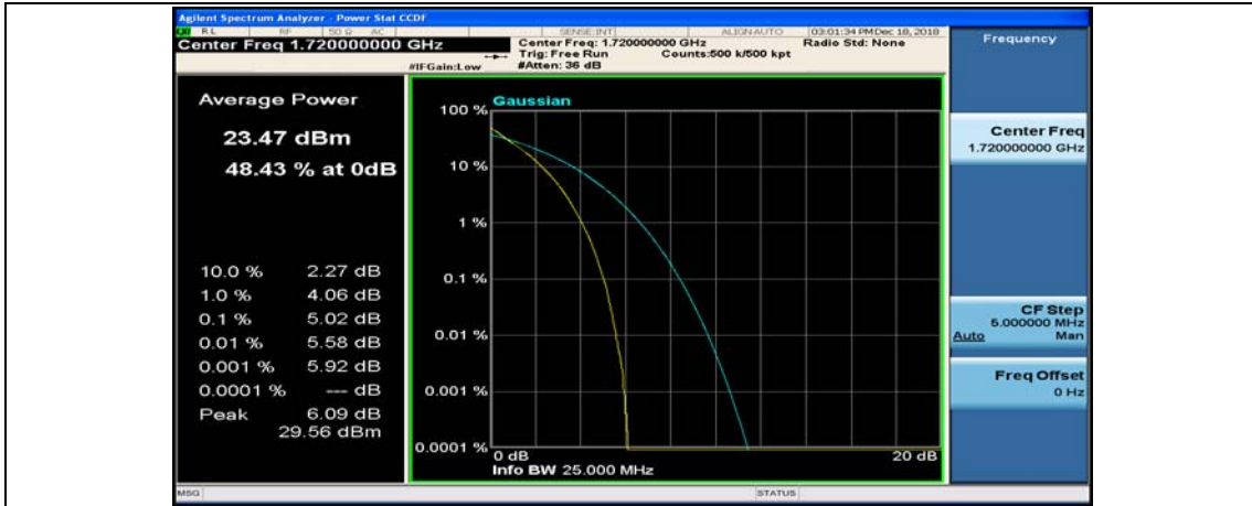
(Channel Bandwidth:20 MHz)_MCH_QPSK_1RB#0
