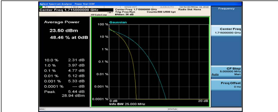
Channel Bandwidth: 10 MHz_MCH_QPSK_1RB#0
