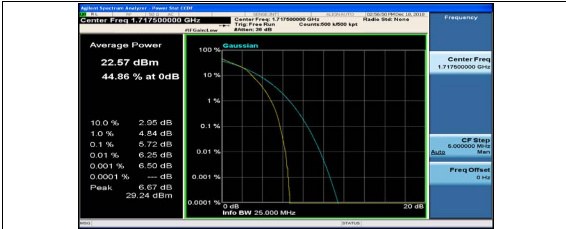
(Channel Bandwidth:15 MHz)_MCH_16QAM_1RB#0
