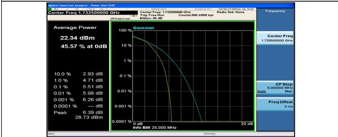
(Channel Bandwidth:15 MHz)_MCH_16QAM_75RB#0
