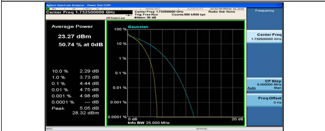
Channel Bandwidth: 10 MHz_MCH_QPSK_25RB#25
