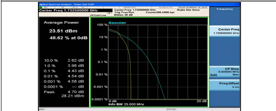
(Channel Bandwidth:20 MHz)_MCH_16QAM_1RB#99
