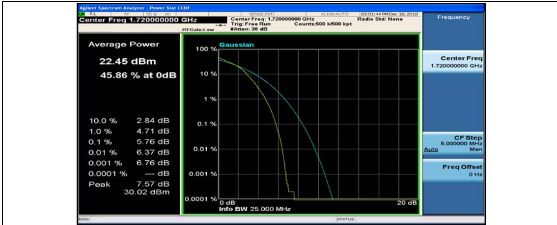
(Channel Bandwidth:20 MHz)_MCH_16QAM_1RB#0
