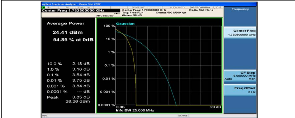
(Channel Bandwidth:15 MHz)_MCH_QPSK_1RB#74
