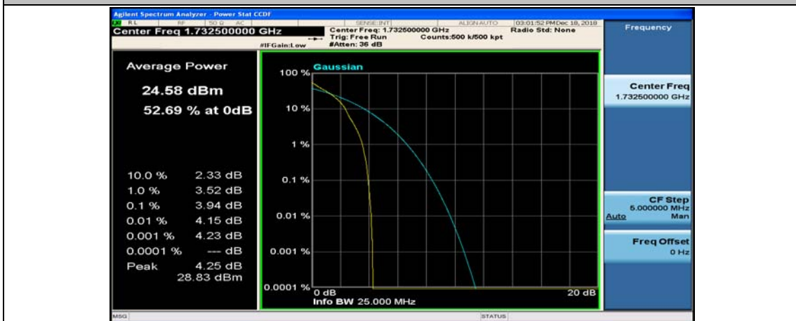
(Channel Bandwidth:20 MHz)_MCH_QPSK_1RB#49
