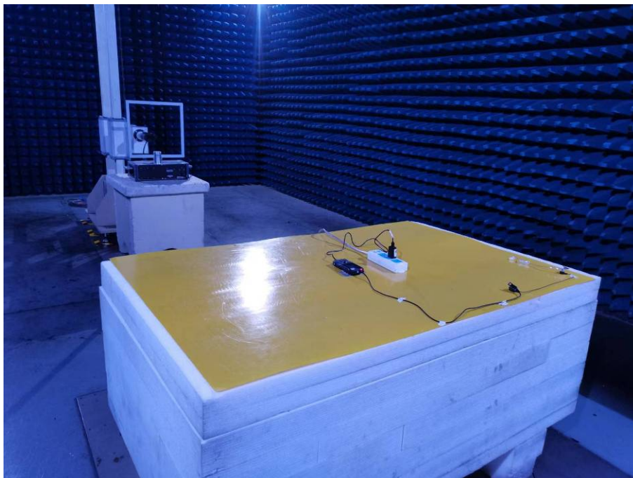
Photo of Radiated Emission Measurement (9kHz-30MHz)
