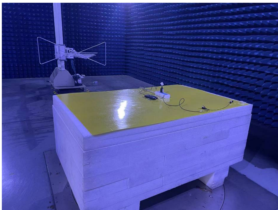
Photo of Radiated Emission Measurement (30MHz-1GHz)
