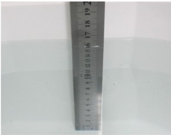
Liquid Height for Head SAR
