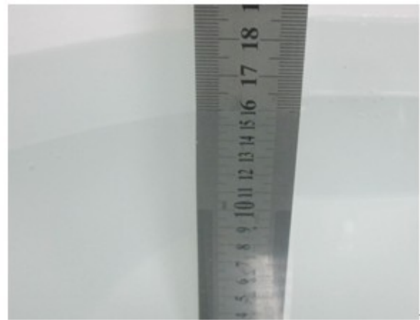
Liquid Height for Body SAR
