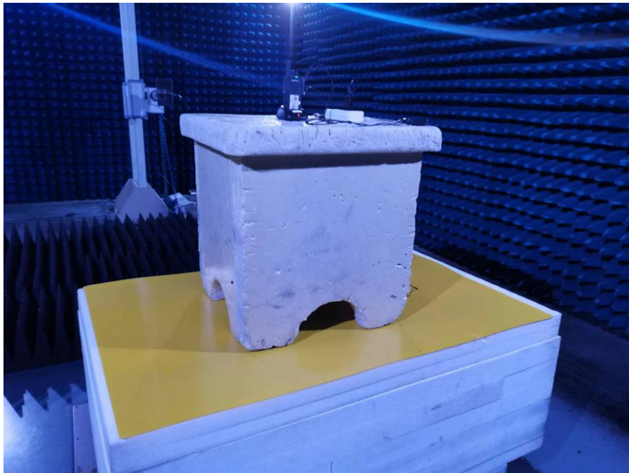
Photo of Radiated Emission Measurement (Above 1G)
