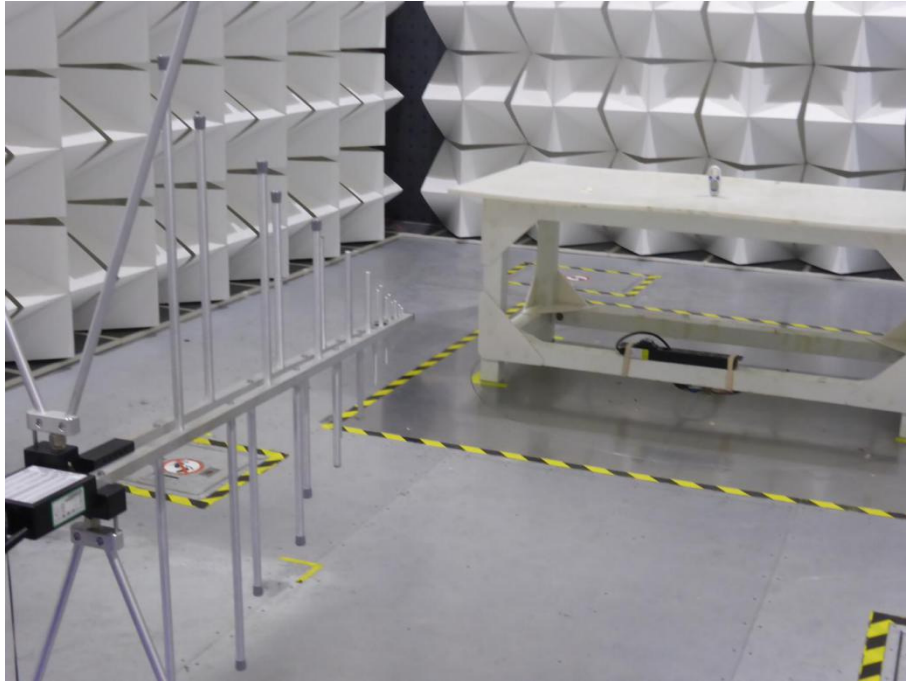
Radiated spurious emission Test Setup-1 (Below 1GHz)
