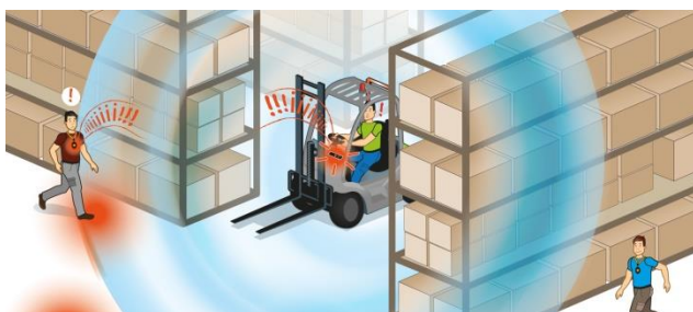
Figure 5 The PROXIPI system installed on a machine detects pedestrians and other machines. When a badge enters the detection area of the machine then, depending on the sensitivity defined on the badge, the alert is triggered.
