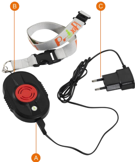
Figure 15 Charging the badge and location of the charging indicator.
