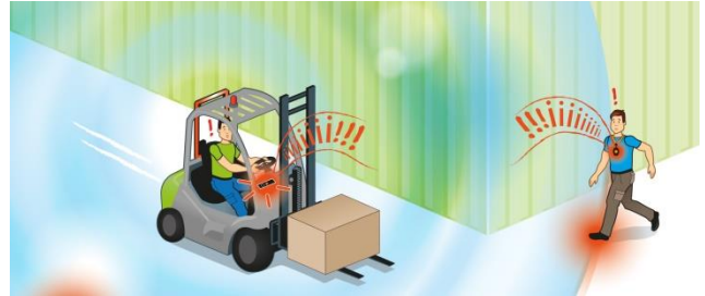
Figure 6 The pedestrian badge detects machines within specified radii. When the badge enters the detection area of the machine then, depending on the sensitivity defined on the badge, the alert is triggered.
