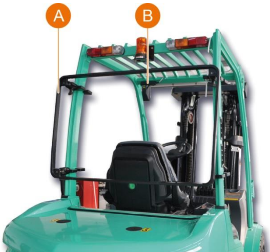
Figure 8 The main components of the PROXIPI system installed on the machine.
