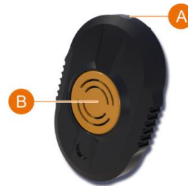
Figure 14 Pressing the acknowledgement button (B) stops the audible alarm (B) and the vibrator. The visual alarm (A) continues to flash.
