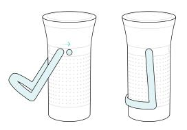
2. Expand the kickstand to funnel clean air at an angle
