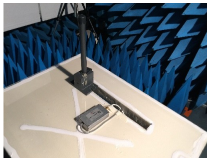
General Test setup for anechoic chamber and OATS in Axis XY:
