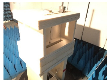
General Test setup for anechoic chamber and OATS in Axis XY:
