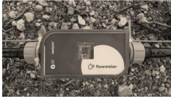
Figure 8. Flow sensor installed on a \varnothing 16mm flexible hose using barbed connectors (not included).
