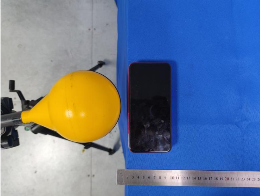
Test Position E(2cm) - Exposure photo from side edge surface-Right(TM10)
