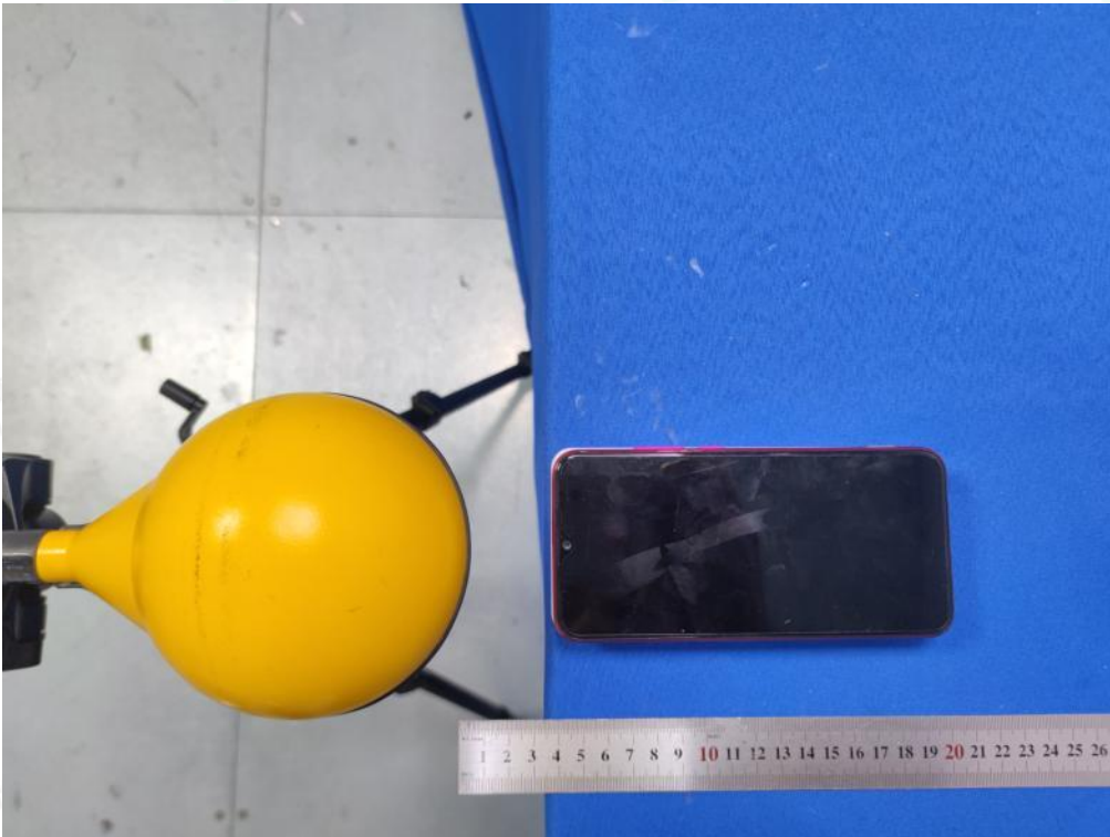
Test Position B(4cm) - Exposure photo from side edge surface-Rear(TM10)
