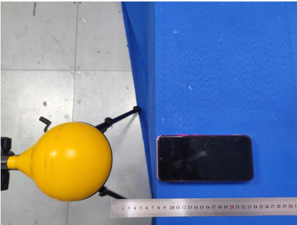
Test Position B(8cm) - Exposure photo from side edge surface-Rear(TM10)
