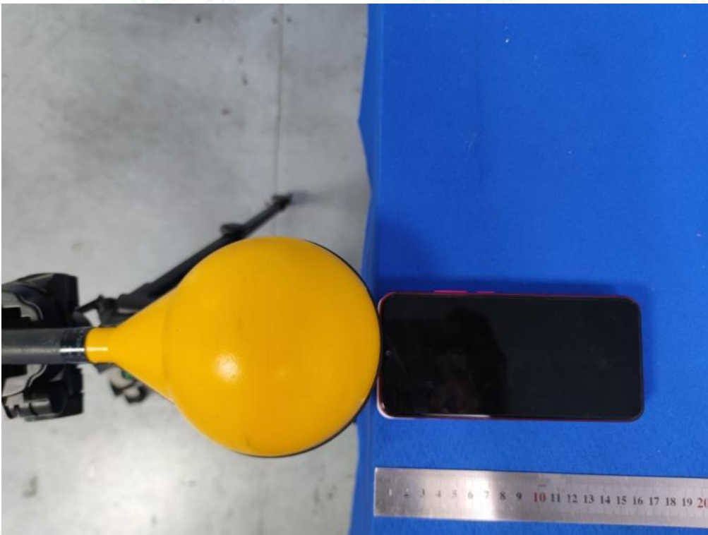
Test Position D(0cm) - Exposure photo from side edge surface-Front(TM10)
