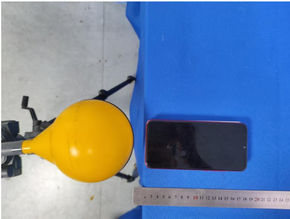
Test Position D(2cm) - Exposure photo from side edge surface-Front(TM10)
