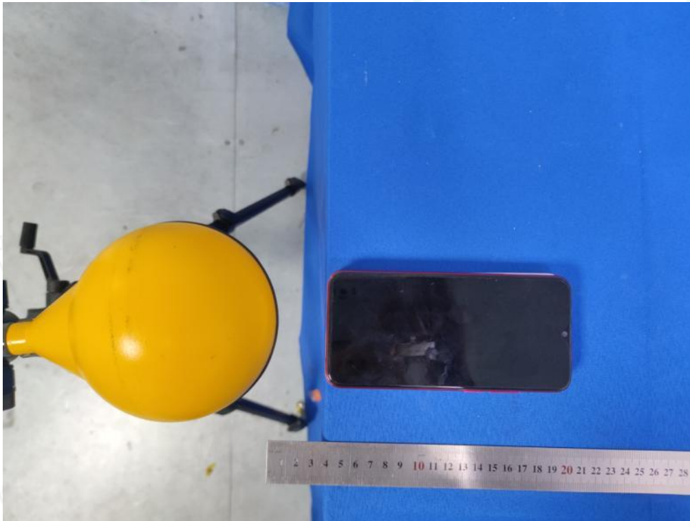
Test Position D(4cm) - Exposure photo from side edge surface-Front(TM10)
