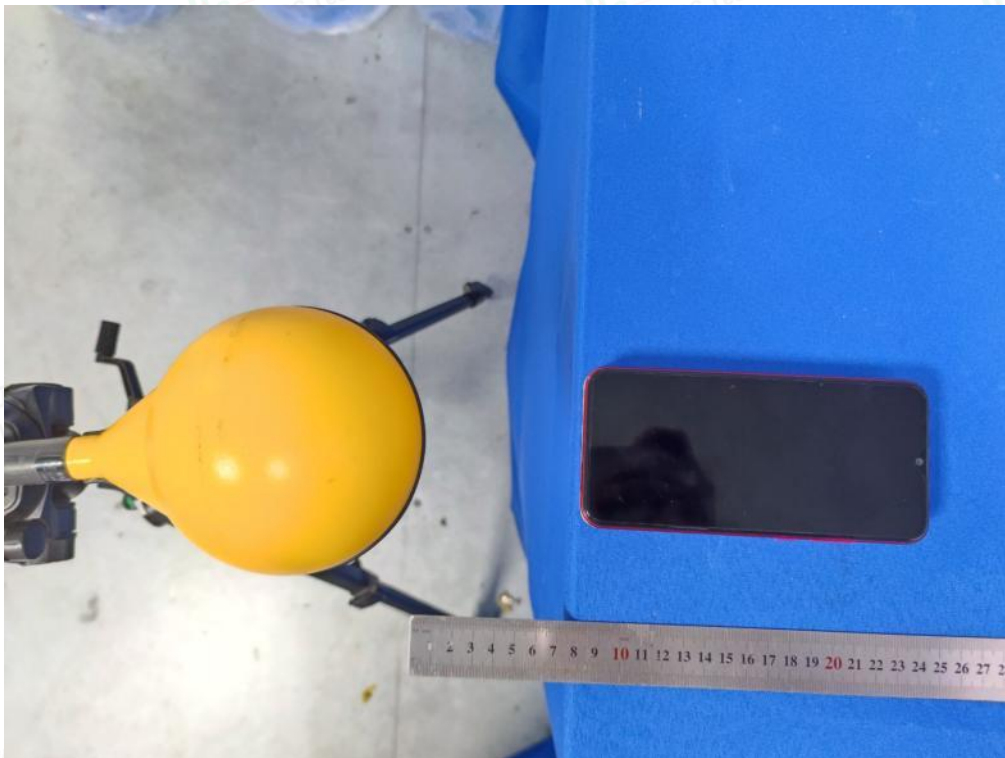
Test Position D(8cm) - Exposure photo from side edge surface-Front(TM10)
