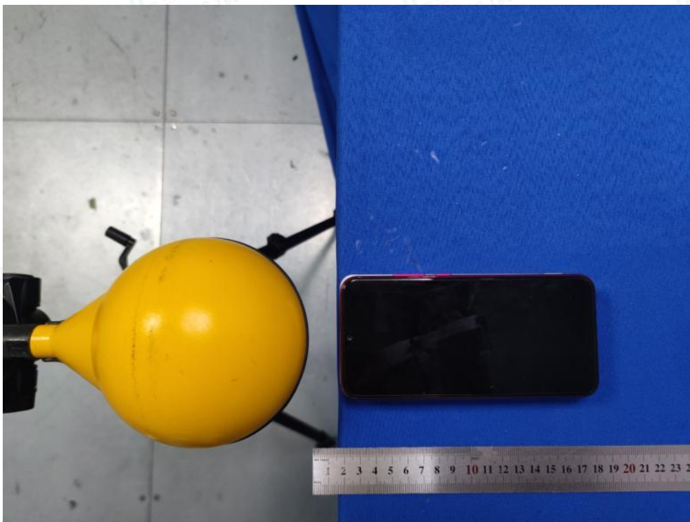
Test Position B(2cm) - Exposure photo from side edge surface-Rear(TM10)
