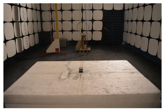
3. Radiated emission (9KHz-30MHz)
