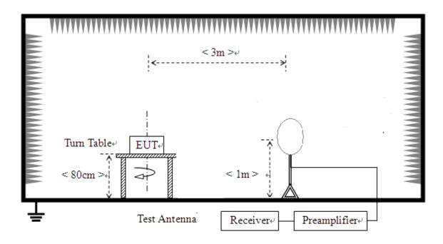
2) For radiated emissions from 30MHz to1GHz
