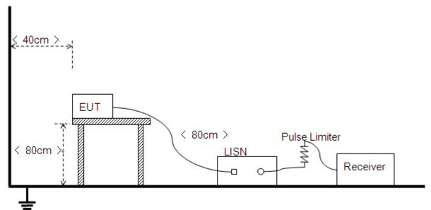
The Table-top EUT was placed upon a non-metallic table 0.8m above the horizontal metal reference ground plane. EUT was connected to LISN and LISN was connected to reference
