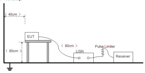
The Table-top EUT was placed upon a non-metallic table 0.8m above the horizontal metal reference ground plane. EUT was connected to LISN and LISN was connected to reference
