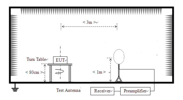
2) For radiated emissions from 30MHz to1GHz
