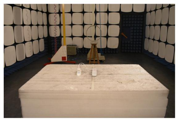
3. Radiated emission (9KHz-30MHz)
