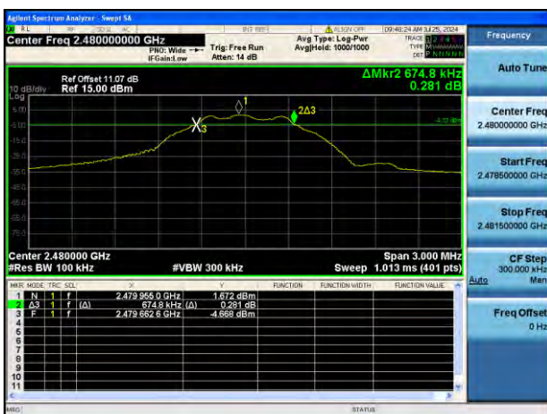
GFSK (BLE 1Mbps) HIGH CHANNEL
