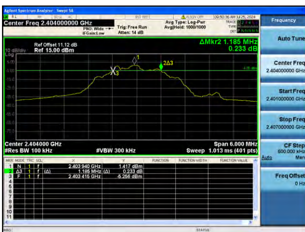
GFSK (BLE 2Mbps) LOW CHANNEL
