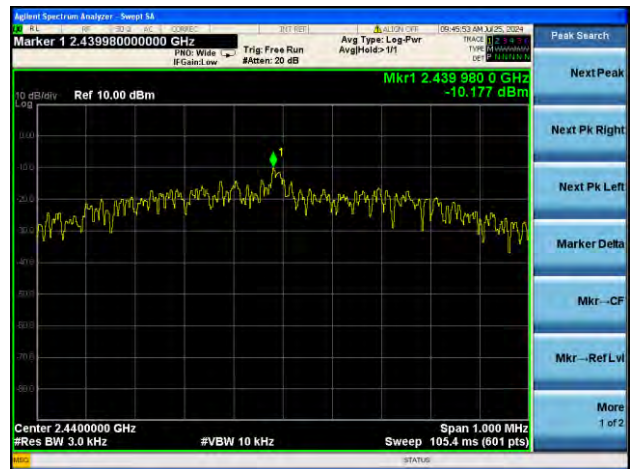
GFSK (BLE 1Mbps) MIDDLE CHANNEL
