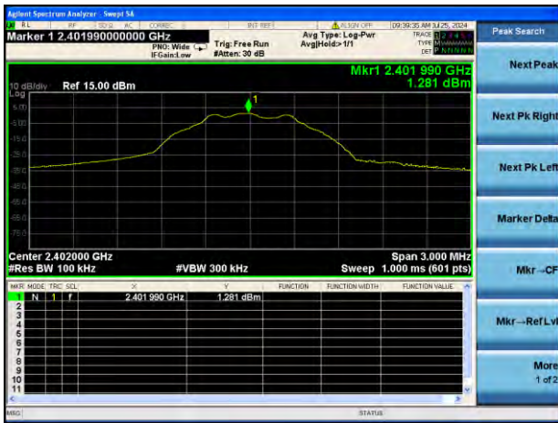
GFSK (BLE 1Mbps) LOW CHANNEL, CARRIER LEVEL
