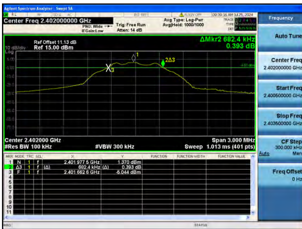
GFSK (BLE 1Mbps) LOW CHANNEL
