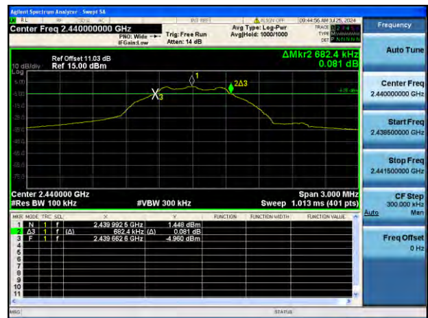
GFSK (BLE 1Mbps) MIDDLE CHANNEL
