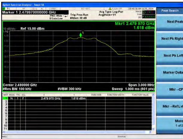
GFSK (BLE 1Mbps) HIGH CHANNEL, CARRIER LEVEL
