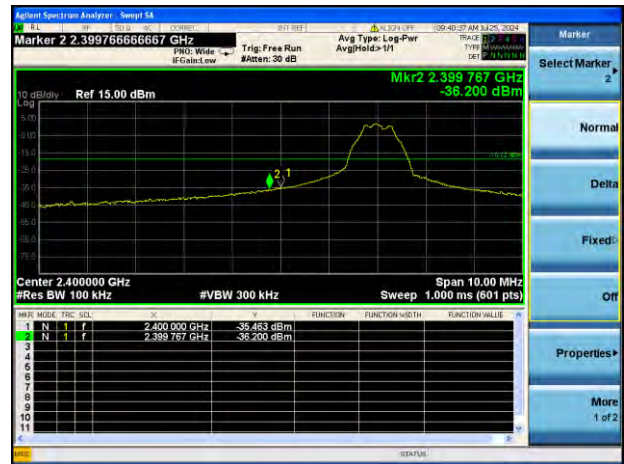
GFSK (BLE 1Mbps) HIGH CHANNEL, BAND EDGE
