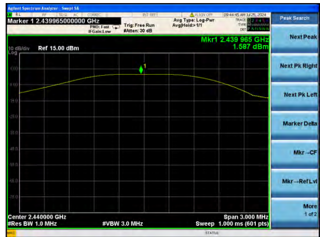
GFSK (BLE 1Mbps) MIDDLE CHANNEL
