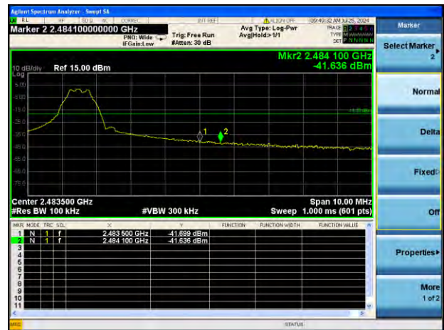
GFSK (BLE 1Mbps) HIGH CHANNEL, BAND EDGE
