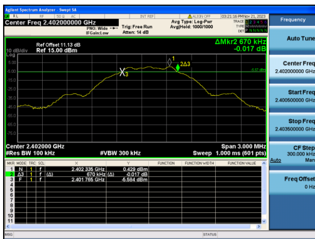
GFSK (BLE 1Mbps) LOW CHANNEL
