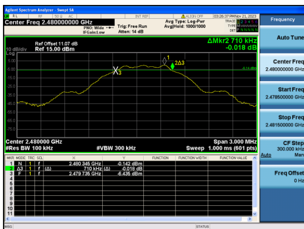
GFSK (BLE 1Mbps) HIGH CHANNEL
