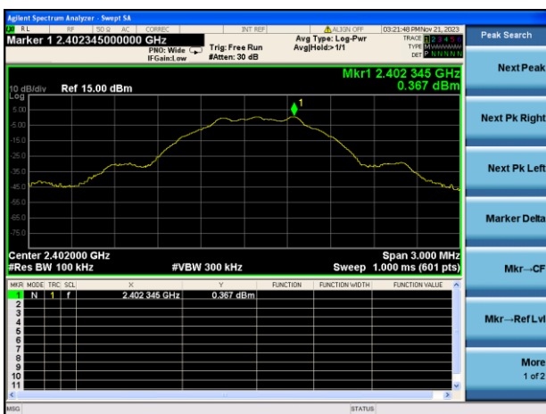
GFSK (BLE 1Mbps) LOW CHANNEL, CARRIER LEVEL
