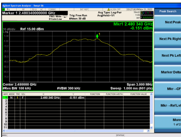
GFSK (BLE 1Mbps) HIGH CHANNEL, CARRIER LEVEL
