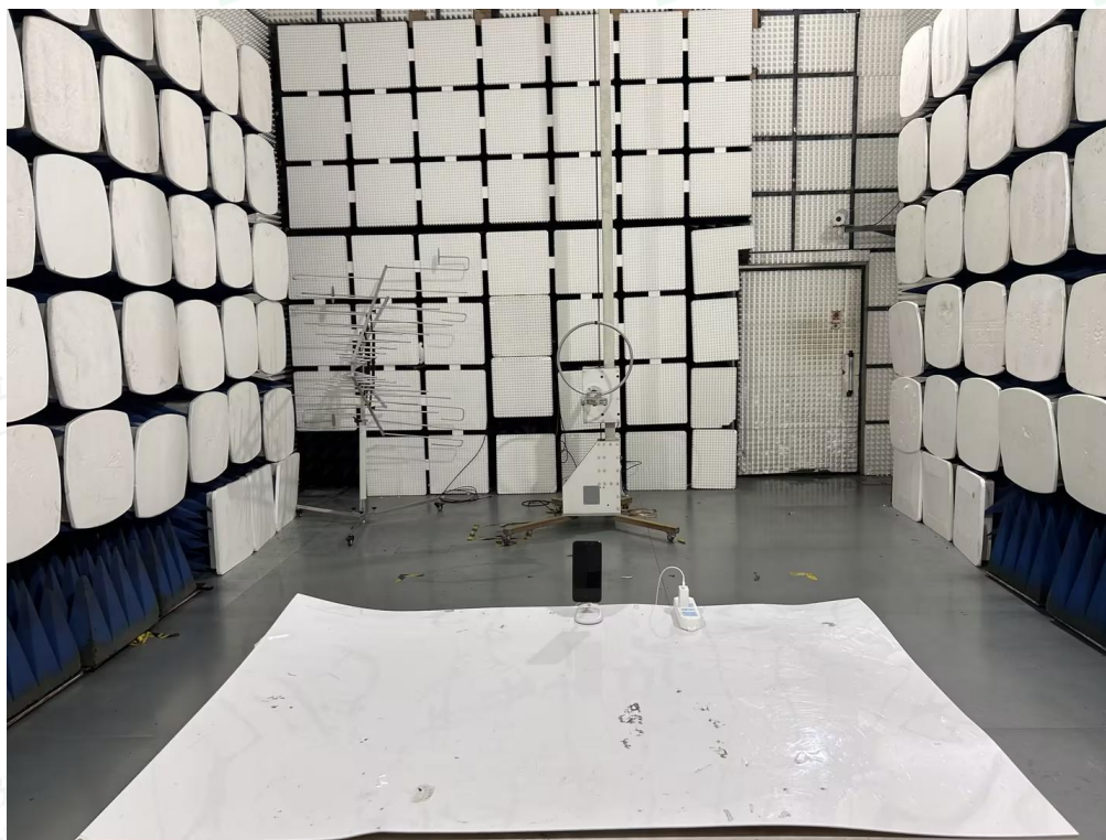
Radiated Emission below 30MHz-AC adapter charge mode
