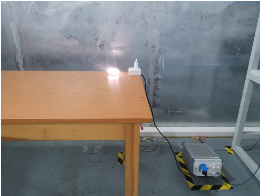
Photo of Power Line Conducted Measurement
