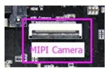
Board support 1400W pixel Mipi camera, Installed in jp26 socket, the electrical definition of the socket is as follows:
