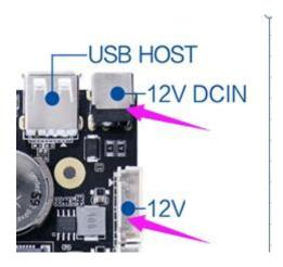
Power socket interfaces are defined as follows, can use power panel power supply, the socket specifications is 6 pin 2.54 mm spacing.
