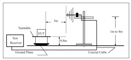
(c) For radiated emissions above 1000MHz
