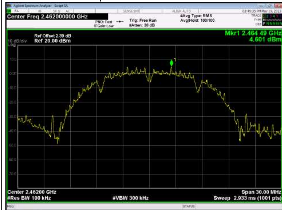
Tx. Spurious NVNT b 2462MHz Emission
