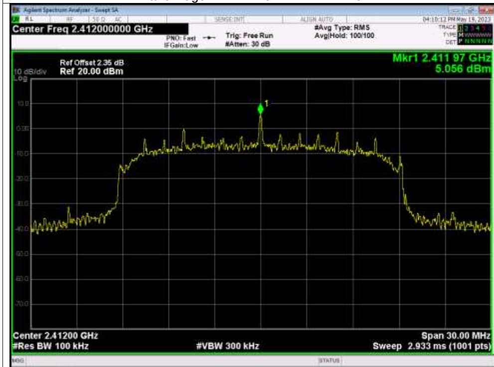
Band Edge NVNT n20 2412MHz Emission
