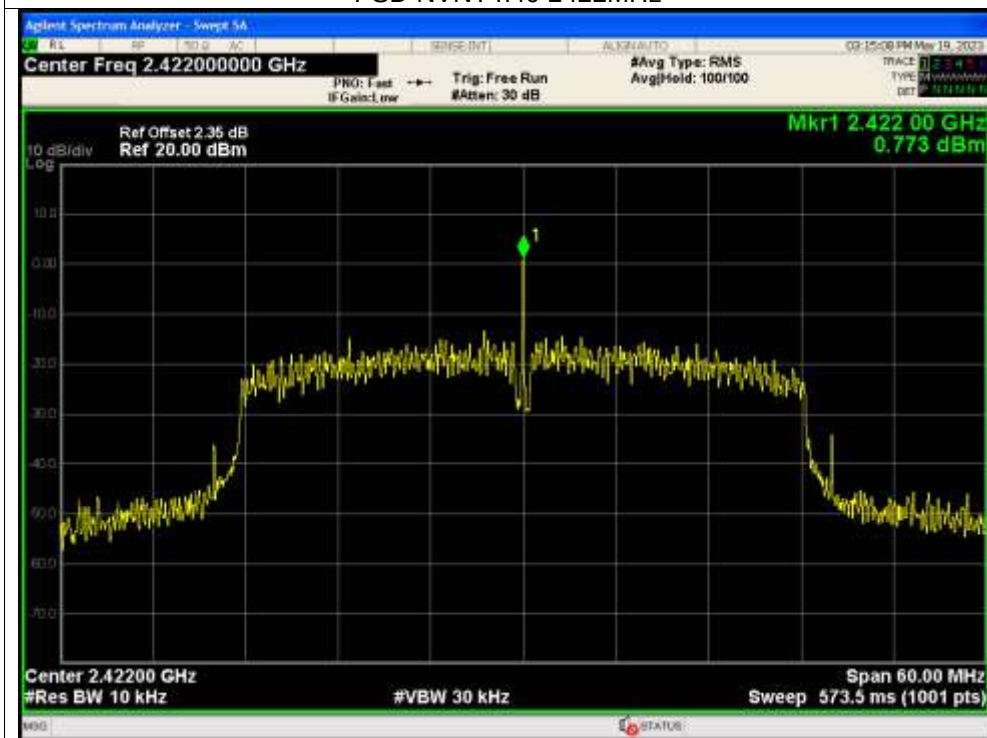
PSD NVNT n40 2422MHz
