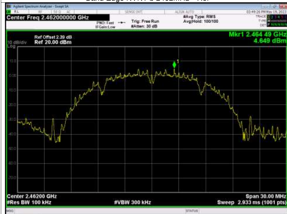
Band Edge NVNT b 2462MHz Emission
