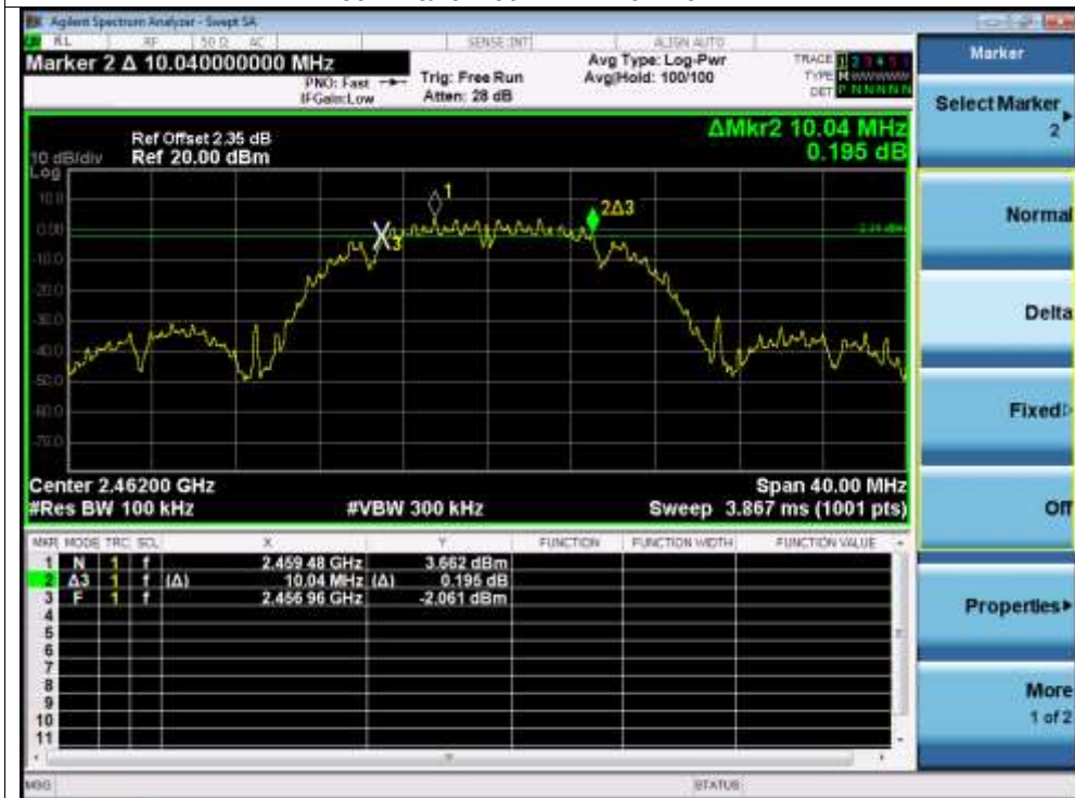
-6dB Bandwidth NVNT g 2412MHz
