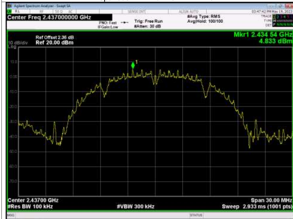
Tx. Spurious NVNT b 2437MHz Emission
