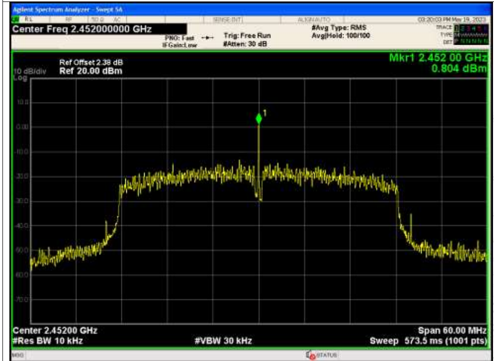
PSD NVNT n40 2452MHz
