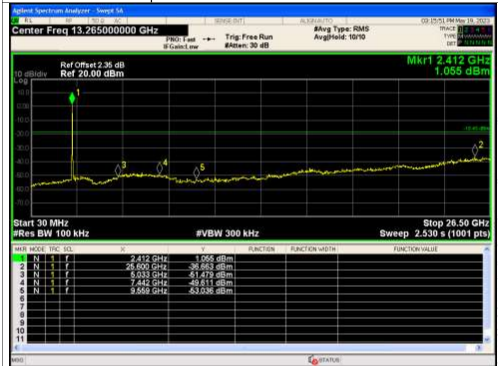
Tx. Spurious NVNT n40 2422MHz Emission
