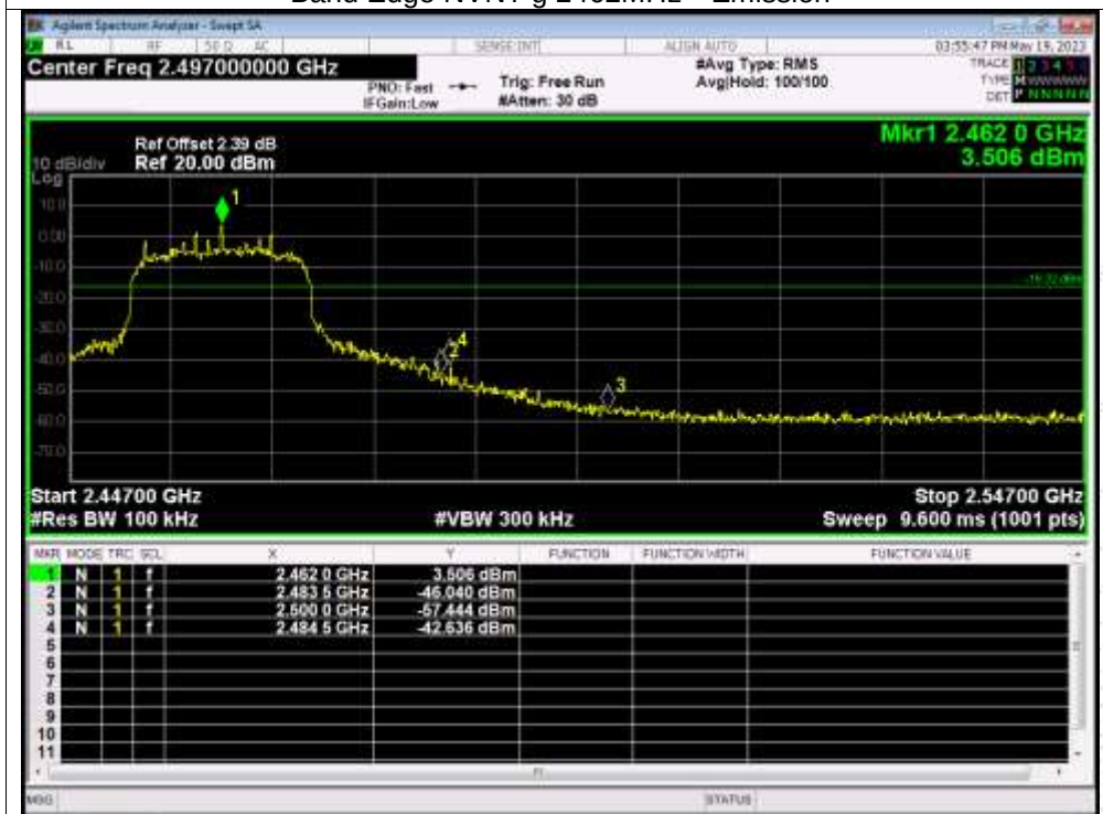
Band Edge NVNT g 2462MHz Emission
