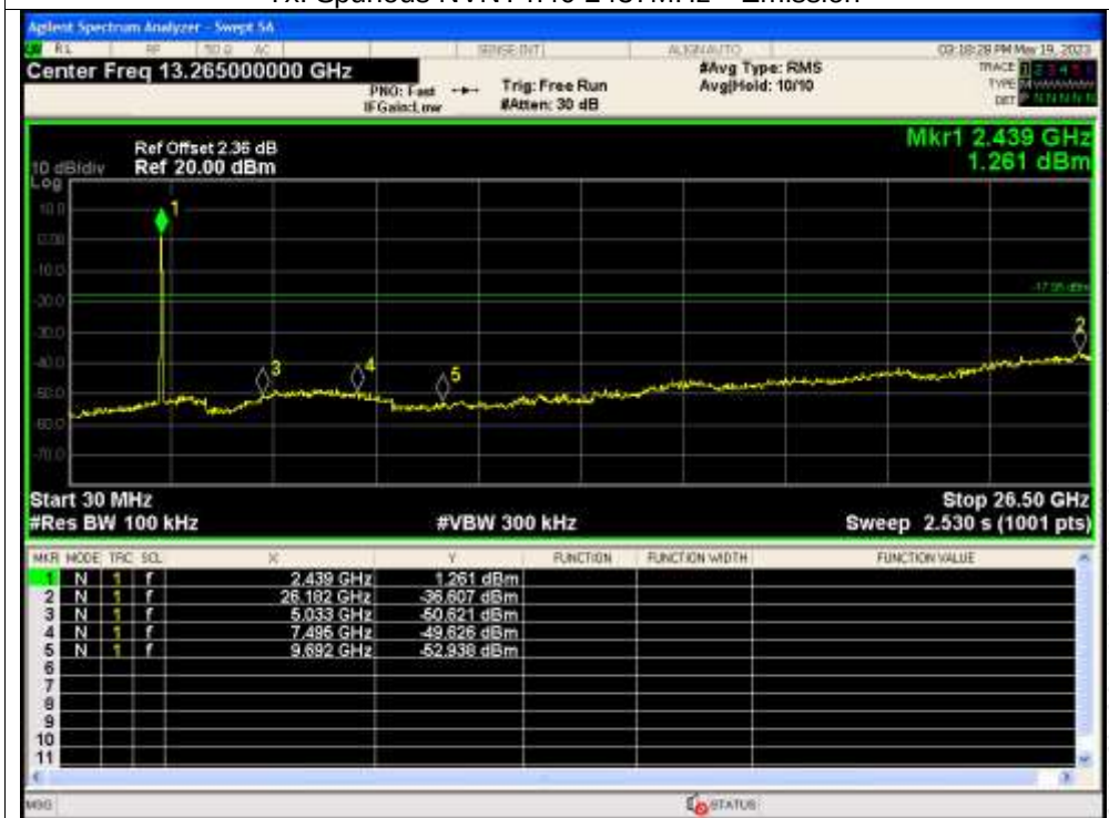
Tx. Spurious NVNT n40 2437MHz Emission
