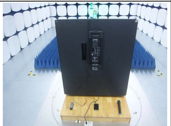
Radiated Emissions Test Setup Above 1GHz
