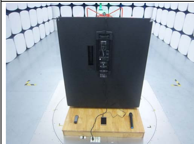
Radiated Emissions Test Setup Below 1GHz
