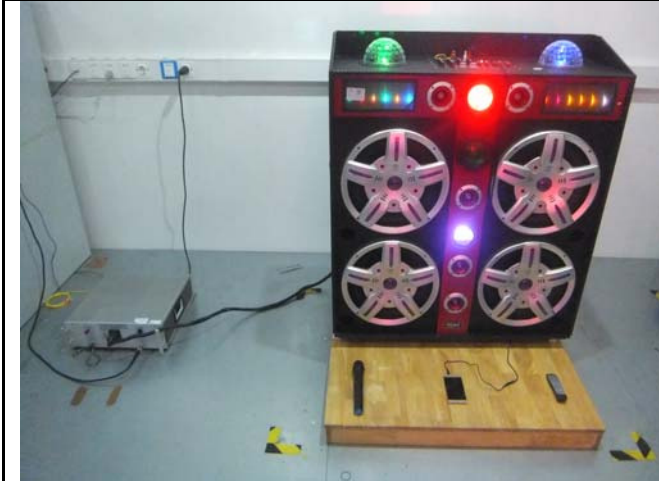
Conducted Emissions Test Setup Front View
