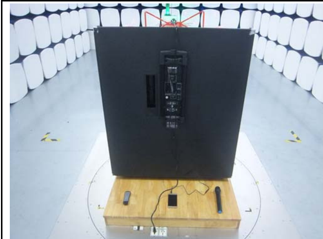
Radiated Emissions Test Setup Below 1GHz
