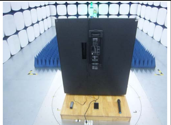
Radiated Emissions Test Setup Above 1GHz
