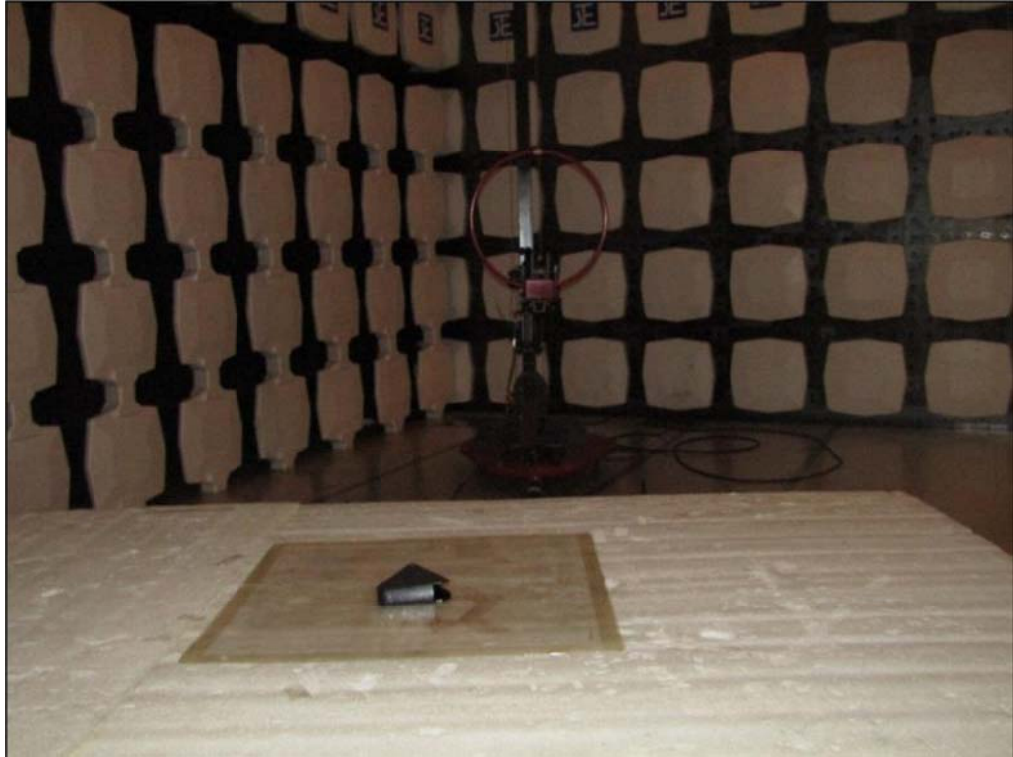
Measurement of Radiated Emission Test Set Up
