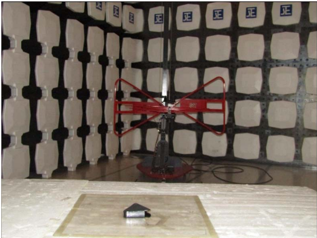
Measurement of Radiated Emission Test Set Up
