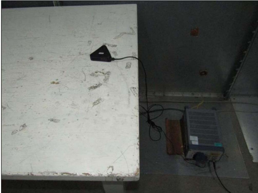
Measurement of Conducted Emission Test Set Up
