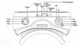
Power key: Long press (5 seconds) the key to achieve power on / off, short press to achieve the sleep / wake-up action, longer press (10 seconds) to forcibly power off;
