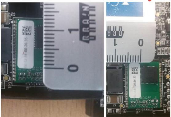
As shown in the above photos, RMBLE-M5 is mounted on the host PCB. RMBLE-M5 label does not have big space so that only Mac address/QR code and product name are printable. There is not enough space to print out FCC and IC ID. Even the small font size of FCC and IC ID can be printable but invisible.
