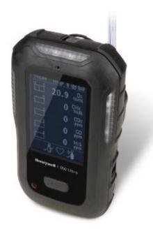
BW Ultra is a portable multi-gas detector for use in hazardous location. Maximum 5 sensors are possible and 02, CO, H2S and LEL sensors are default while 5th sensor is various per customer's selection. BW Ultra is designed to operate with the lithium-ion battery pack and the specific charging adaptor is only available. BW Ultra is featured with Bluetooth Low Energy so that user can use a designated mobile application.
