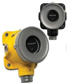
Sensepoint XRL is a single sensor fixed gas detector, which supports the following interfaces dependent on the model – Analogue output (4-20 mA), Digital output (Modbus RTU) and Mobile output (Bluetooth Low Energy). Sensepoint XRL is available for the detection of the following gases:
