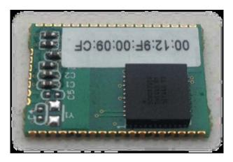
RMBLE-M5 uses a radio technology called frequency-hopping spread spectrum (FHSS). The transmitted data are divided into packets and each packet is transmitted on one of the 40 channels, channel spacing 2 MHz. The first channel starts at 2402 MHz and continues up to 2480 MHz. RMBLE-M5 can coexist with DSSS based Wi-Fi very well due to different transmit protocol.
