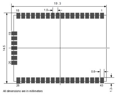
Please don't place GND plane in the keep-out area, and minimize the area metal traces occupied in the area. It is recommended to have a 0.4 mm gap (T) between the module's upper surface and the plastic housing.
